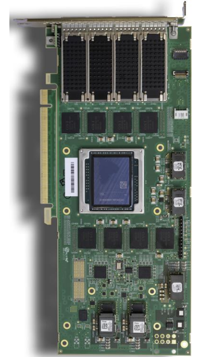
FPGA custom board for SW development
